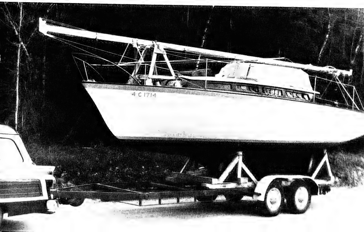
A Mobjack class centerboard boat can easily be trailed by a compact auto (top), while a special cradle is required for keel type boats such as the Amphibi-Con (bottom)
